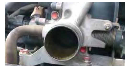
BEFORE (Throttle body condition after 60,000 km)
